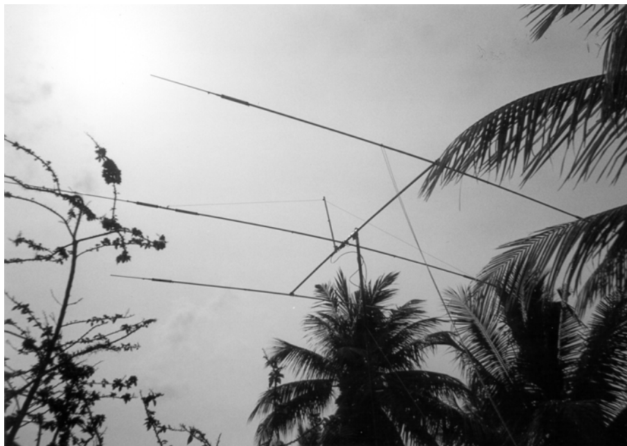
The Cushcraft A3WS beam for 12 and 17m, with an extended driven element for 30m, was raised between the palm trees and rotated by pulling round the rope attached to the reflector.
